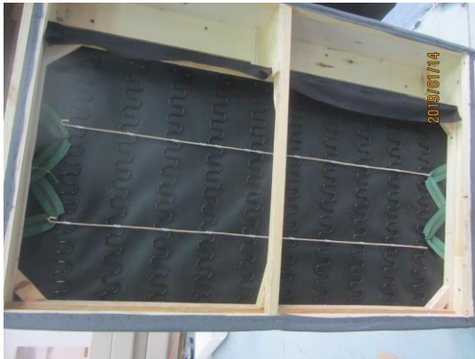
Solid pine for spring rail, size: 38 x 28mm, 10pcs springs
